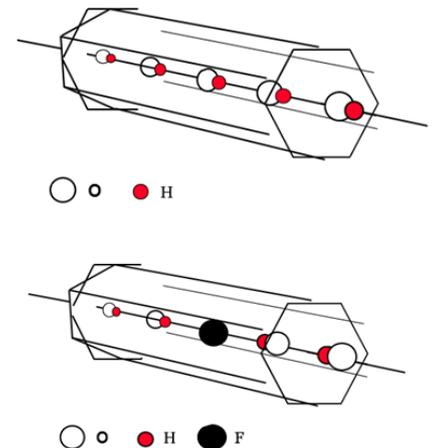
Figure 1: The hexagonal apatite structure with hydroxyl ions and fluoride ions [2].
